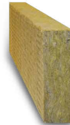
MW Mineralwolle \lambda_d = 0.036 \text{ W/(mK)} Euroklasse A1
